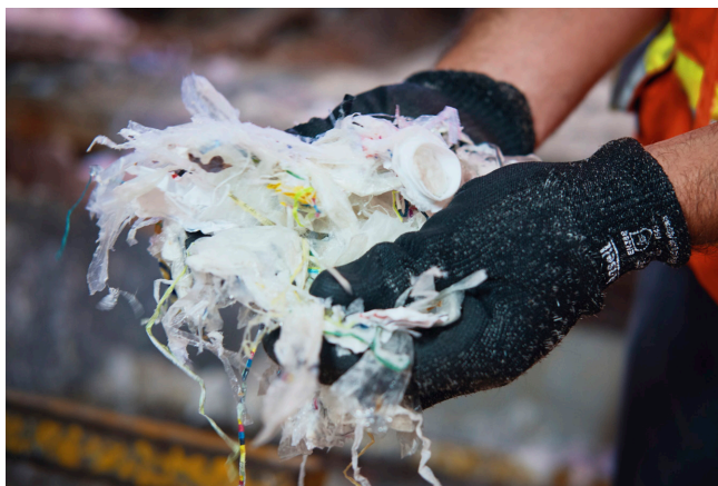
Polyethylene and aluminum components of cartons separated from the fibre
