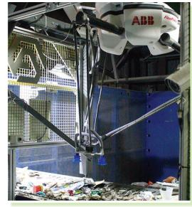
When fully operational, the robot can pick up to 60 or more cartons per minute. Through artificial intelligence (AI), everything learned about identifying cartons can be transferred to other systems.
