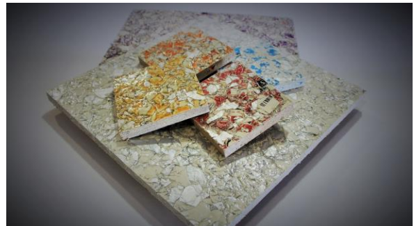
ReWall converts cartons into high-performance, sustainable building materials through its low-energy, eco-friendly recycling technology. Photo Credit: ReWall Company
