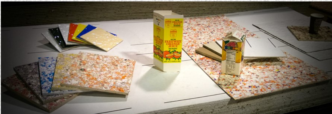
About 30 cartons make up a single 2'x2' ReWall ceiling tile. Source: The ReWall Company - www.rewallsolutions.com
